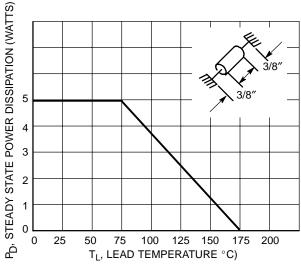
Figure 5. Steady State Power Derating
