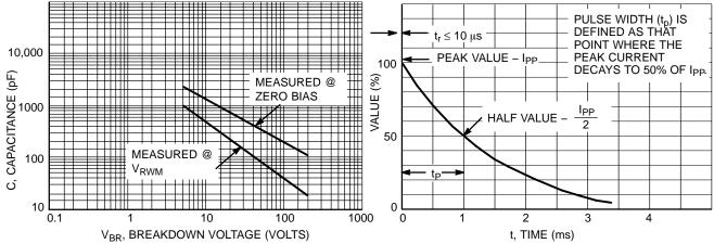
Figure 3. Capacitance versus Breakdown Voltage
