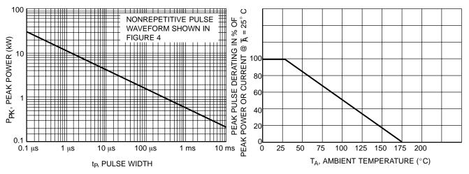
Figure 1. Pulse Rating Curve
