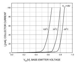
Figure 5. Base-Emitter On Voltage
