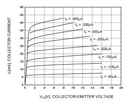
Figure 1. Static Characteristic
