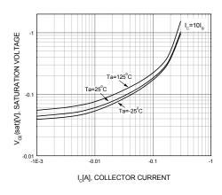
Figure 4. Collector-Emitter Saturation Voltage
