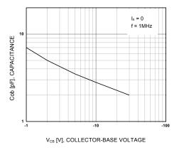
Figure 6. Collector Output Capacitance
