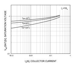
Figure 3. Base-Emitter Saturation Voltage
