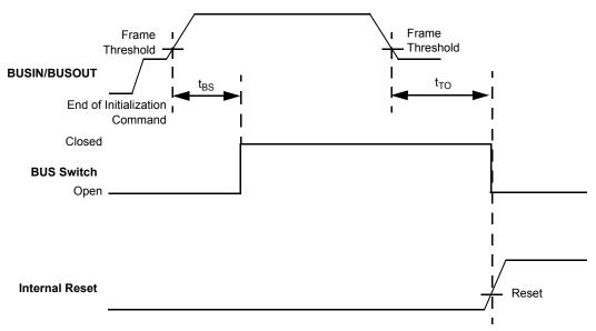
Figure 4. Bus Switch and Reset Timing
