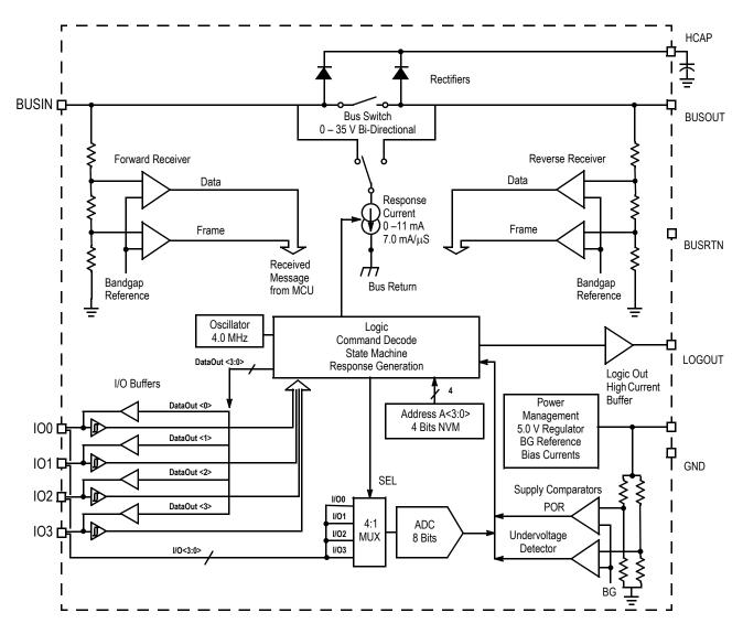
Figure 2. 33793 Simplified Internal Block Diagram
