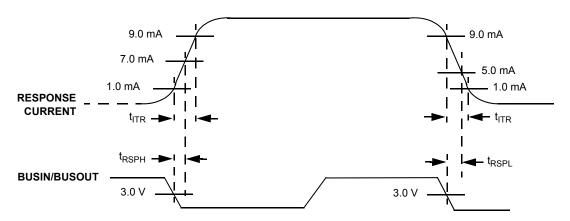
**Figure 5. Response Current Timing**
