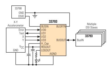
Figure 1. 33793 Simplified Application Diagram
