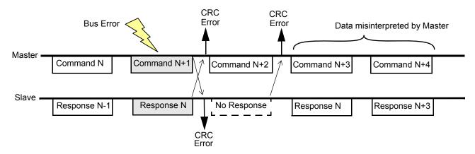
Figure 7. Bus Traffic With Receive Errors (Master Reads Incorrect Data)
