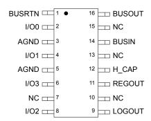
Figure 3. 33793 Pin Connections
