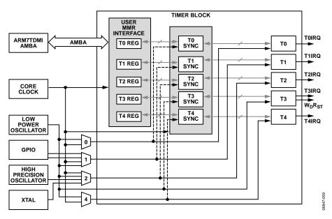
Figure 32. Timer Block Diagram
