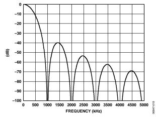
Figure 21. Typical Digital Filter Response at  $f_{ADC} = 1.0 \text{ kHz}$ (ADCFLT = 0x0007)
