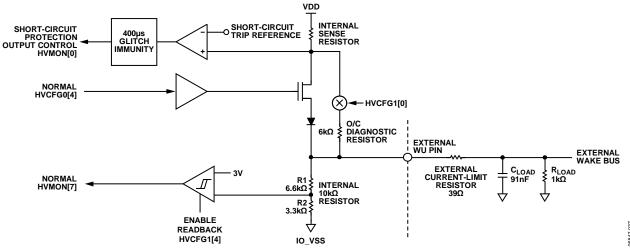
Figure 41. WU Circuit, Block Diagram
