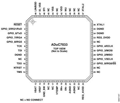
Figure 7. Pin Configuration
