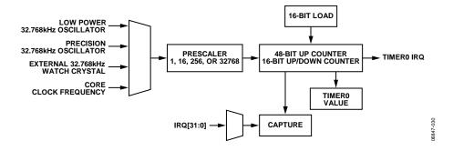
Figure 34. Timer0 Block Diagram
