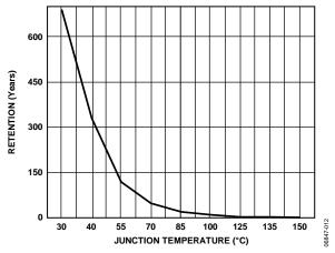
Figure 14. Flash/EE Memory Data Retention
