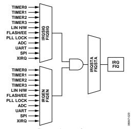
Figure 31. Interrupt Structure
