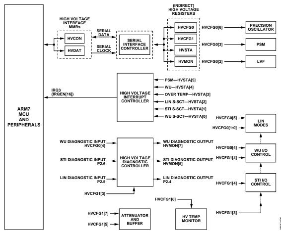
Figure 40. High Voltage Interface, Top Level Block Diagram
