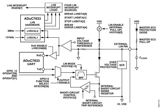
Figure 45. LIN I/O, Block Diagram
