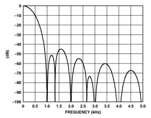
Figure 22. Modified Sinc3 Digital Filter Response at f<sub>ADC</sub> = 1.0 kHz (ADCFLT = 0x0087)
