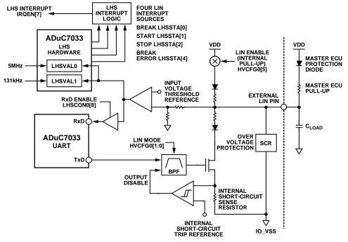
Figure 52. BSD I/O Hardware Interface
