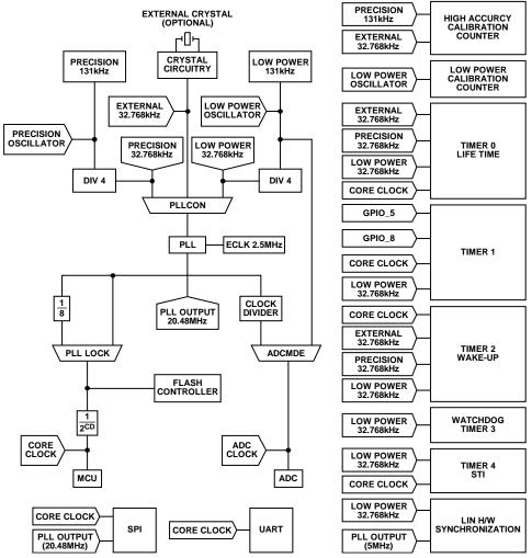
Figure 29. ADuC7033 System Clock Generation
