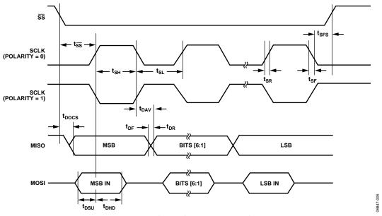
Figure 4. SPI Slave Mode Timing (PHASE Mode = 1)
