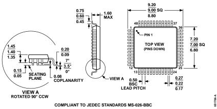
Figure 60. 48-Lead Low Profile Quad Flat Package [LQFP] (ST-48) Dimensions shown in millimeters
