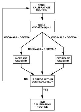
Figure 30. OSCOTRM Calibration Routine
