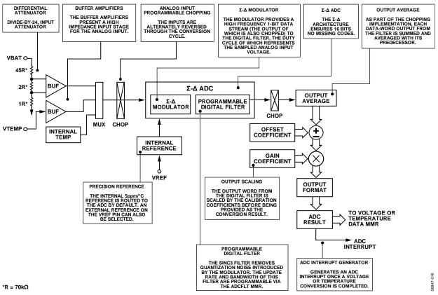
Figure 18. Voltage/Temperature ADC, Top Level Overview
