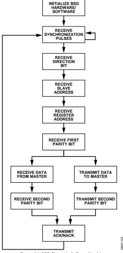
Figure 56. BSD Slave Node State Machine
