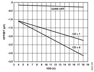
Figure 10. ADC Current Channel Offset vs. Supply @ 25°C
