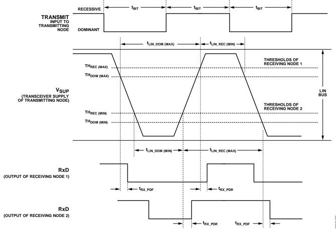
Figure 6. LIN 2.0 Timing Specification
