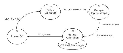
Figure 6. Clock Generator Power-up/Run State Diagram
