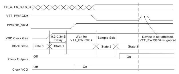
Figure 5. VTT\_PWRGD# Timing Diagram
