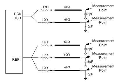
Figure 7. Single-ended Load Configuration
