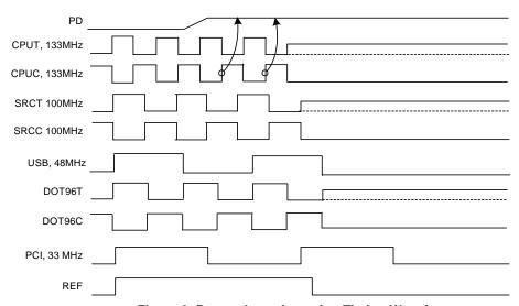
Figure 3. Power-down Assertion Timing Waveform
