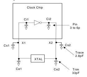
Figure 2. Crystal Loading Example
