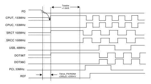
Figure 4. Power-down Deassertion Timing Waveform
