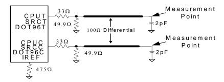
Figure 8. 0.7V Single-ended Load Configuration
