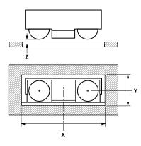
X is the width of the window, Y is the height of the window, and Z is the distance from the HSDL-3200 to the back of the window.
