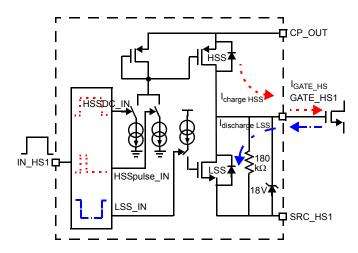
Figure 5. High-Side Gate Driver Functional Schematic
