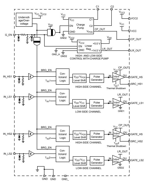
Figure 2. 33883 Simplified Internal Block Diagram
