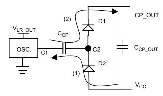
Figure 8. Charge Pump Basic Circuit
