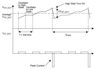
Figure 11. Simplified C<sub>CP\_OUT</sub> Current and Voltage Waveforms
