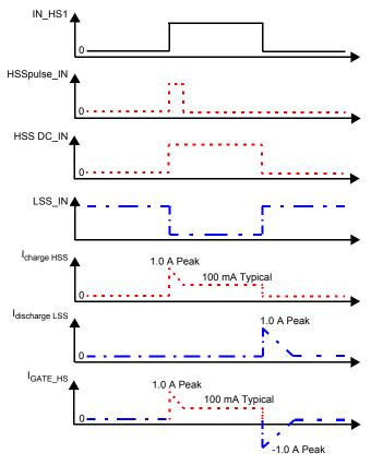
**Note** GATE\_HS is loaded with a 100 nF capacitor in the chronograms. A smaller load will give lower peak and DC charge or discharge currents.
