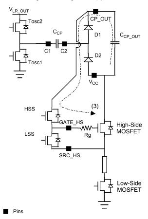
Figure 9. High-Side Gate Driver
