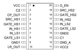
Figure 3. 33883 20-SOICW Pin Connections
