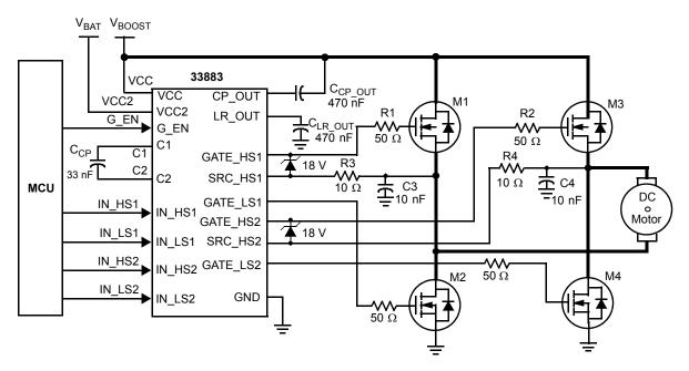
Figure 14. Application Schematic with External Protection Circuit
