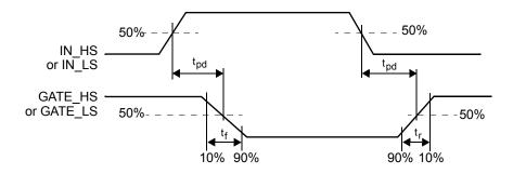
Figure 4. Timing Characteristics
