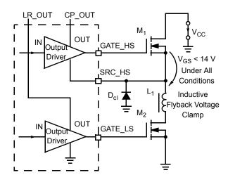
Figure 12. Gate Protection and Flyback Voltage Clamp
