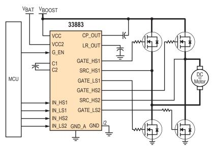
Figure 1. 33883 Simplified Application Diagram
