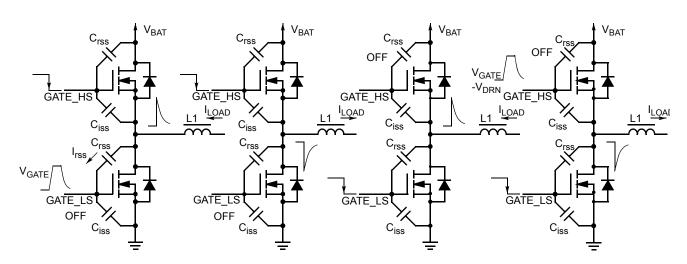
Driver Requirement: Low Resistive Gate-Source Path During OFF-State Driver Requirement: Low Resistive Gate-Source Path During OFF-State. High Peak Sink Current Capability Driver Requirement: High Peak Sink Current Capability Driver Requirement: Low Resistive Gate-Source Path During OFF-State
