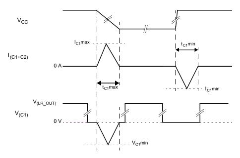
Figure 13. Limits of C1 Current and Voltage with Large Values of dV/dt
