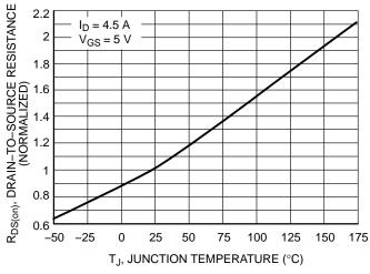
Figure 5. On–Resistance Variation with Temperature
