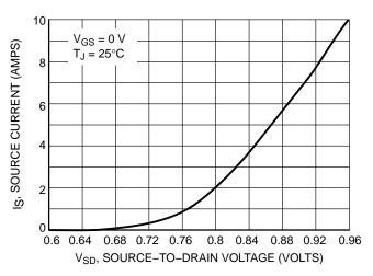
Figure 10. Diode Forward Voltage versus Current
