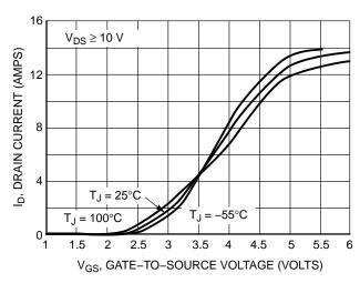
**Figure 2. Transfer Characteristics**
