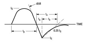
Figure 14. Diode Reverse Recovery Waveform
