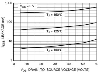
Figure 6. Drain-to-Source Leakage Current versus Voltage
