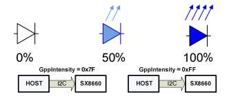
Figure 29 LED control in GPP mode
