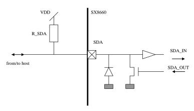
Figure 43 Simplified diagram of SDA
