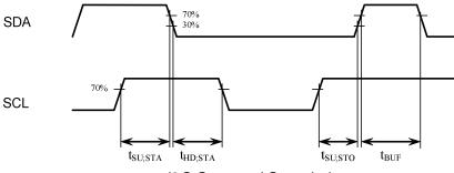
Figure 4 I2C Start and Stop timing
