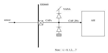
Figure 39 Simplified diagram of CAP0, CAP1,...,CAP7
