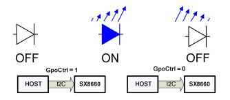
Figure 30 LED Control in GPO mode, Autolight OFF
