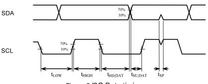
Figure 5 I2C Data timing
