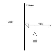
Figure 46 Simplified diagram of VDD
