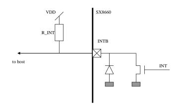
Figure 41 Simplified diagram of INTB
