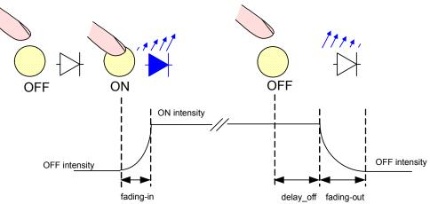
The GPO pin fades in when the associated button is touched and it fades out when it is released. This is shown in Figure 36
