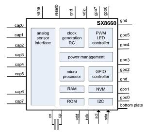
Figure 3 Simplified block diagram of the SX8660
