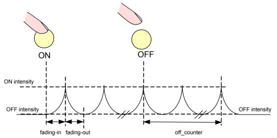
Figure 37 Continuous Fading Mode
