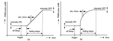
Figure 35 GPO OFF transition (LED fade out), inverted polarity, (a) linear, (b) logarithmic
