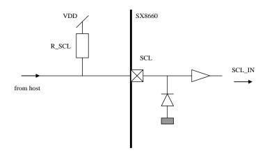
Figure 42 Simplified diagram of SCL
