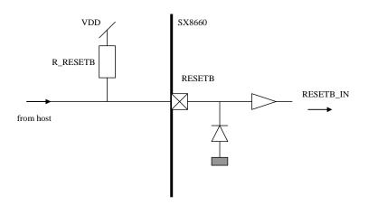
Figure 44 Simplified diagram of RESETB controlled by host
