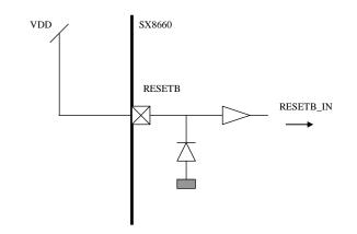
Figure 45 Simplified diagram of RESETB without host control
