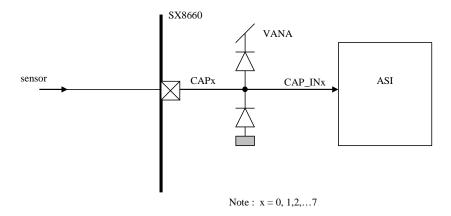
Figure 39 shows the simplified diagram of the CAP0, CAP1,...CAP7 pins.
