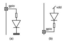
Figure 27 polarity = 1 (a), polarity = 0 (b)
