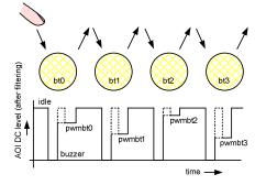
Figure 16 AOI behavior with 0V buzzer state
