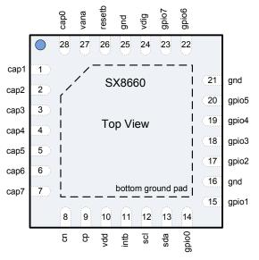
Figure 1 Pinout Diagram
