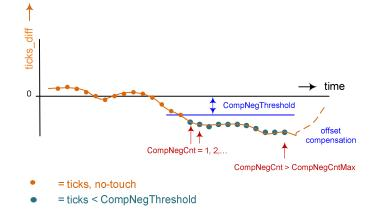
Figure 52 Negative Ticks Offset Compensation Trigger
