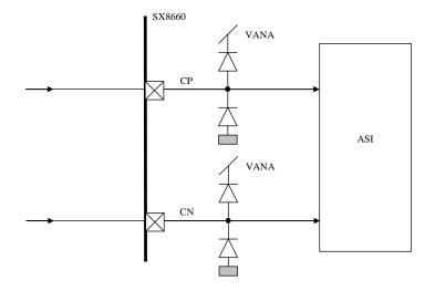
Figure 40 Simplified diagram of CN and CP
