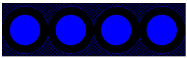
Figure 9 PCB top layer of four sensors for buttons (surrounded by a ground plane)
