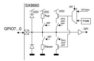
Figure 49 Simplified diagram of GPIO pins
