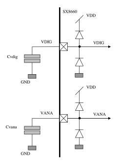
Figure 48 Simplified diagram of VANA and VDIG
