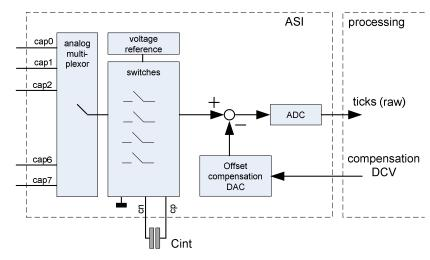
Figure 17 Analog Sensor Interface
