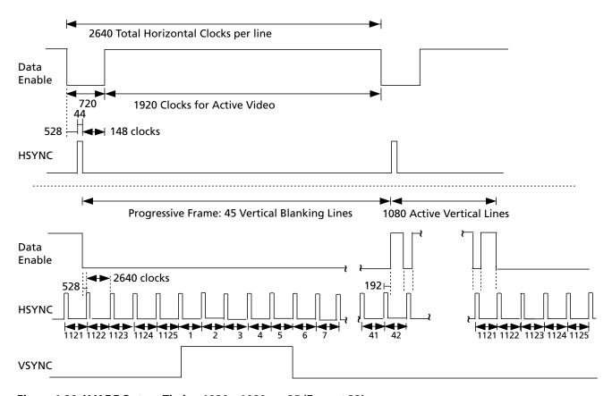
Figure 4-39: H:V:DE Output Timing 1920 x 1080p @ 25 (Format 33)
