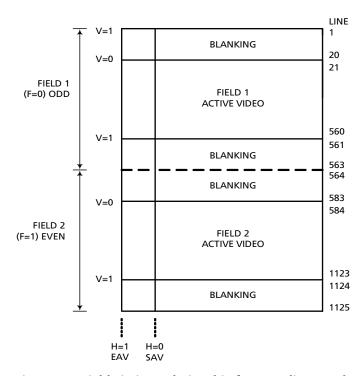
Figure 4-6: Field Timing Relationship for 1080-line Interlaced Systems
