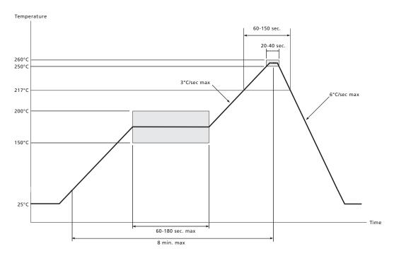
Figure 6-3: Pb-free Solder reflow Profile
