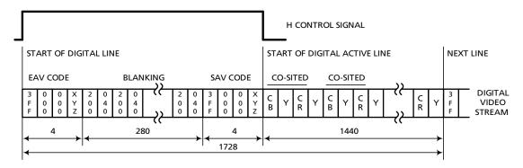
Figure 4-5: Multiplexing 10-bit 4:2:2 YCbCr data for 625 lines at 50Hz
