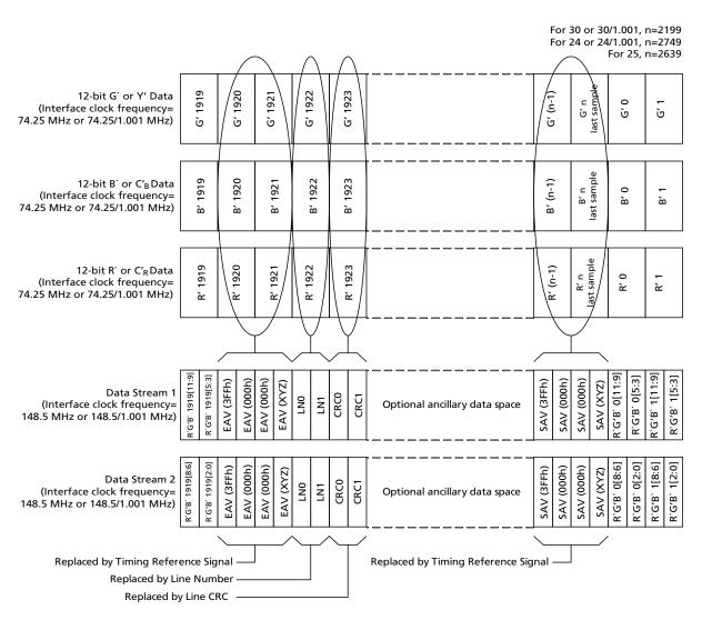
Figure 4-17: Aviia 20-bit Mapping Structure for 1920 x 1080 24/25/30Hz Progressive 4:4:4 (R'G'B' or Y'C' $_B$ C' $_R$ ) 12-bit Signals
