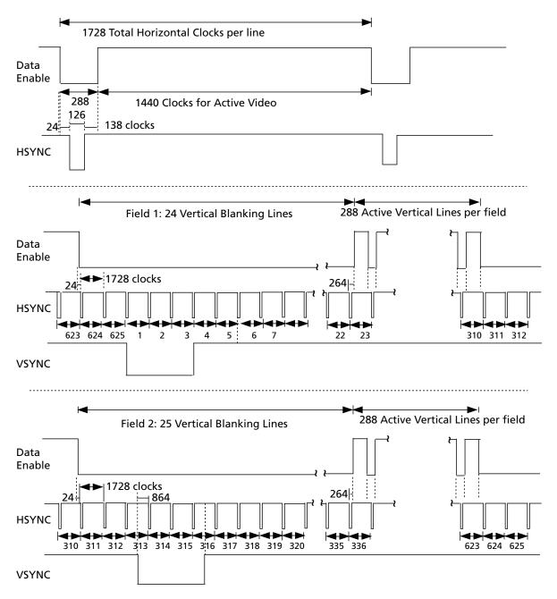
Figure 4-35: H:V:DE Output Timing 720 (1440) x 576 @ 50 (Format 21 & 22)
