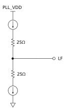
Figure 3-7: Loop Filter (LF)
