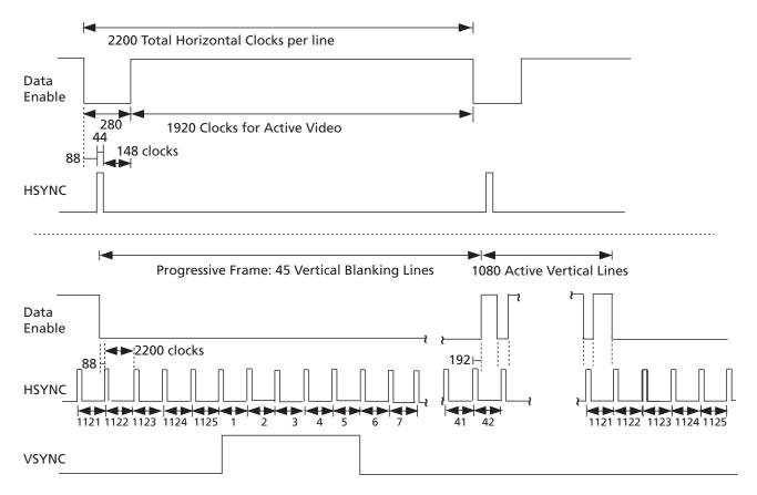
Figure 4-36: H:V:DE Output Timing 1920 x 1080p @ 59.94/60 (Format 16)
