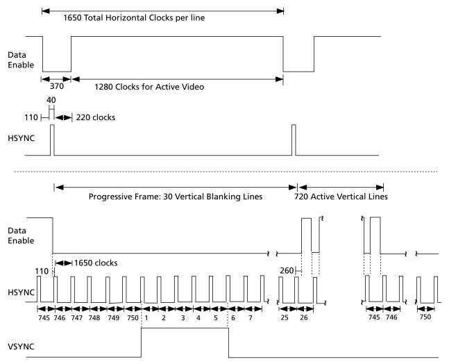
Figure 4-30: H:V:DE Output Timing 1280 x 720p @ 59.94/60 (Format 4)
