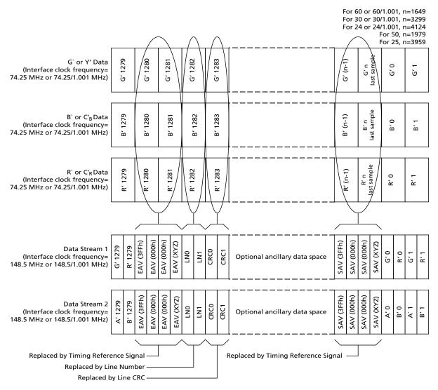
Figure 4-19: Aviia 20-bit Mapping Structure for 1280 x 720 24/25/30/25/60Hz Progressive 4:4:4 (R'G'B' or Y'C' $_B$ C' $_R$ ) 8/10-bit Signals
