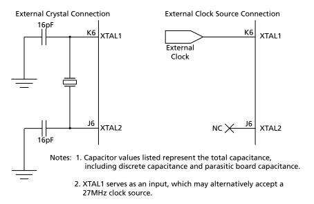
Figure 4-1: 27MHz Clock Sources
