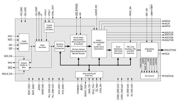
Figure A: GV7601 Block Diagram
