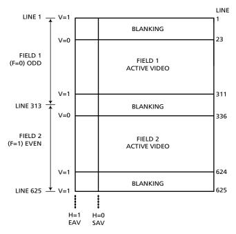
Figure 4-4: Data transmitting with blanking, 625/50Hz
