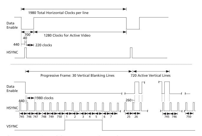
Figure 4-33: H:V:DE Output Timing 1280 x 720p @ 50 (Format 19)
