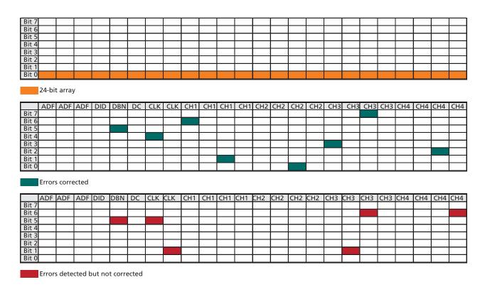
Figure 4-58: ECC 24-bit Array and Examples
