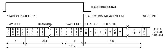
Figure 4-3: Multiplexing 10-bit 4:2:2 YCbCr data for 525 lines at 60Hz
