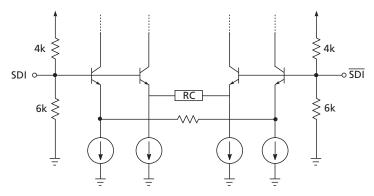
Figure 3-8: Serial Input Equivalent Circuit
