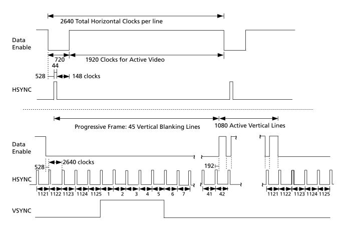
Figure 4-37: H:V:DE Output Timing 1920 x 1080p @ 50 (Format 31)
