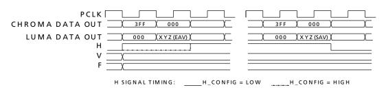
Figure 4-28: H:V:F Output Timing - SD 20-bit Output Mode
