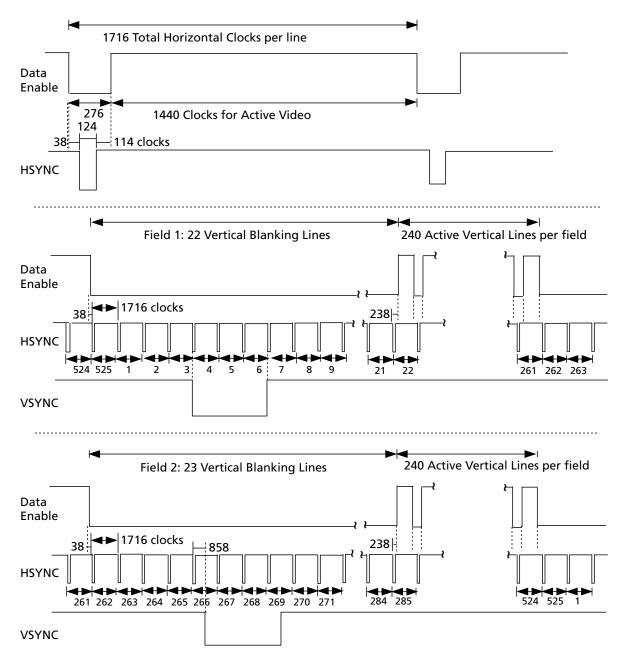
Figure 4-32: H:V:DE Output Timing 720 (1440) x 480i @ 59.94/60 (Format 6 & 7)
