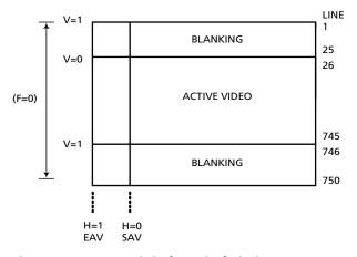
Figure 4-14: 720p Digital Vertical Timing
