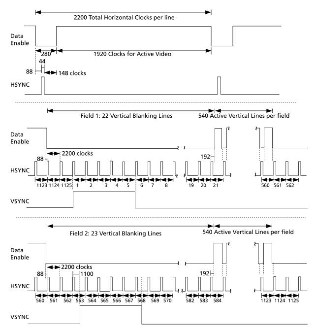
Figure 4-31: H:V:DE Output Timing 1920 x 1080i @ 59.94/60 (Format 5)
