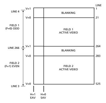
Figure 4-2: Data transmitting with blanking, 525/60Hz
