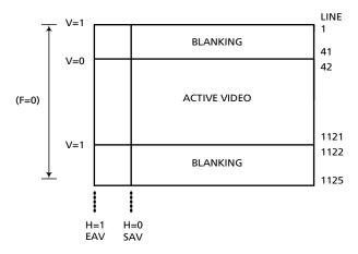
Figure 4-10: Frame Timing Relationship For 1080-line Progressive Systems
