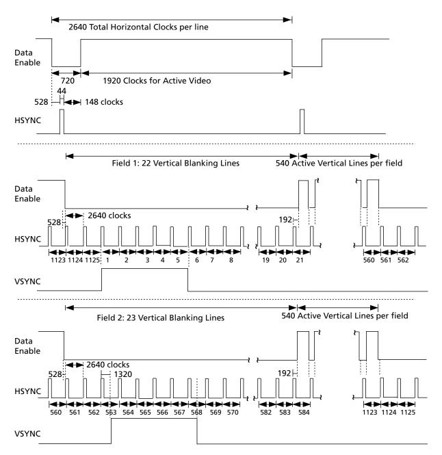
Figure 4-34: H:V:DE Output Timing 1920 x 1080i @ 50 (Format 20)
