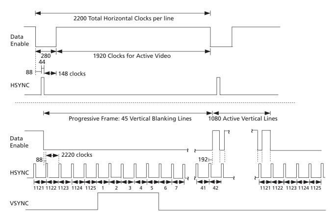
Figure 4-40: H:V:DE Output Timing 1920 x 1080p @ 29.97/30 (Format 34)
