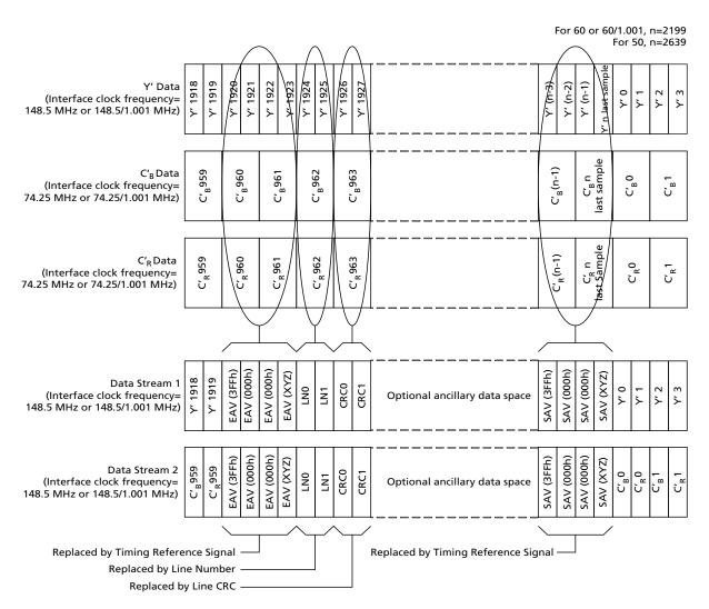
Figure 4-15: Aviia 20-bit Mapping Structure for 1920 x 1080 50/60Hz Progressive 4:2:0 & 4:2:2 ( $Y'C'_BC'_R$ ) 8/10-bit Signals
