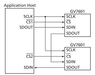
Figure 4-59: GSPI Application Interface Connection
