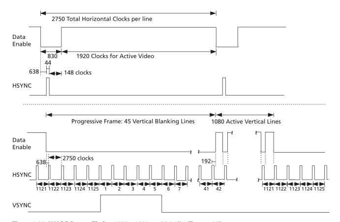
Figure 4-38: H:V:DE Output Timing 1920 x 1080p @ 23.94/24 (Format 32)
