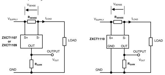
**Figure 1 Basic Application Circuit**
