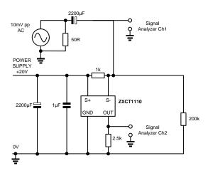
Test circuit for Small signal bandwidth
