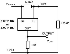
Figure 2. Example Circuit using ZXCT1107/ZXCT1109
