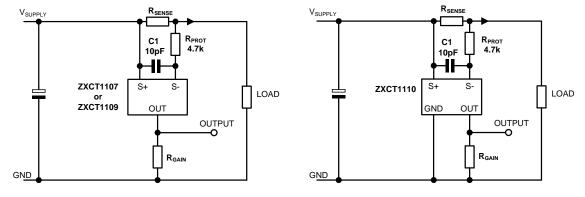
Figure 4 Protection and EMC Filtering
