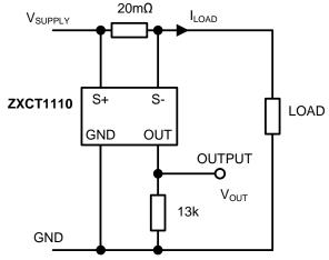
Figure 3 Example Circuit using ZXCT1110
