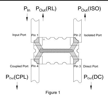
The coupler is excited at the input port with P<sub>in</sub> (watts) of power. Assuming the coupler is not ideal, and that there are no radiation losses, power will exit the coupler at all four ports. Symbolically written, Pout(RL) is the power that is returned to the source because of impedance mismatch, Pout(ISO) is the power at the isolated port, Pout(CPL) is the power at the coupled port, and P<sub>out(DC)</sub> is the power at the direct port.
