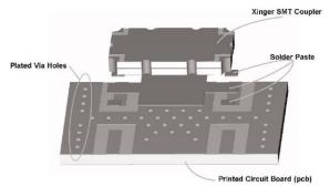
Figure 4: Mounting Features Example
