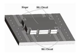
Figure 3: Component Placement
