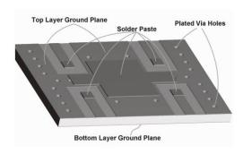
Figure 2: Solder Paste Application
