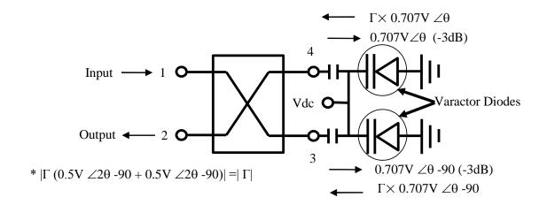
\* The phase angle of the signal exiting port 2 will vary with the phase angle of  $\Gamma$ , which is the reflection angle from the varactor. The varactors must be matched so that their reflection coefficients are equal.
